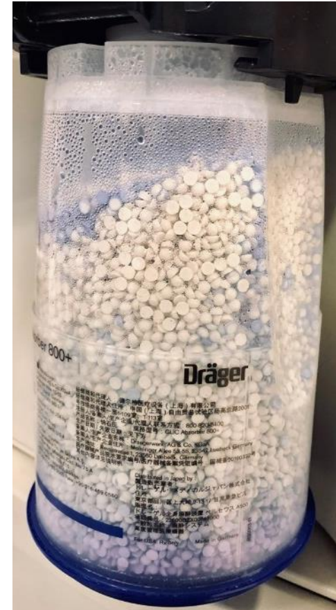
Notice indicator change showing path of gas flow and unreacted absorbent
